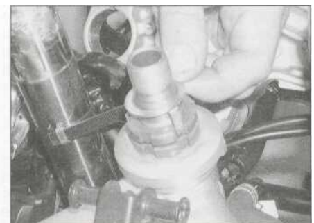
8.7a Remove the tabbed lockwasher ...
