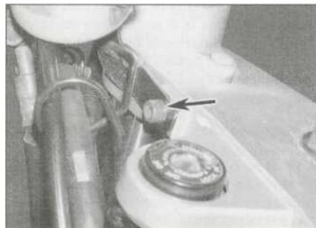
8.3c Unscrew the bolt (arrowed) and displace the cable guide
