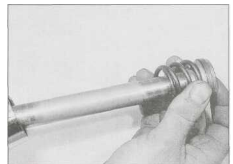
7.38 Withdraw the damper rod and rebound spring from the tube
