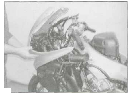
3.20 Draw the fairing forward off the bike
