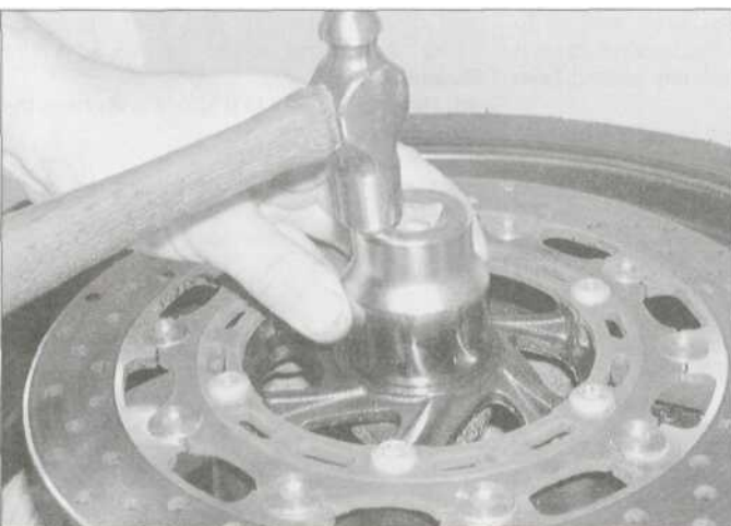
16.10 A socket can be used to drive in the bearing
