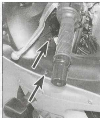
3.7 Each intake duct cover is secured by three screws (arrowed)
