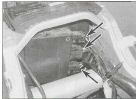
5.3a Disconnect the wiring connectors (arrowed)...
