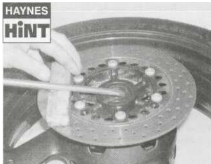
Position a piece of wood against the wheel to prevent the screwdriver shaft damaging it when levering the grease seal out.
