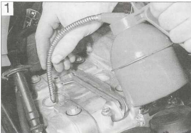
Squirt a drop of motor oil into each cylinder
