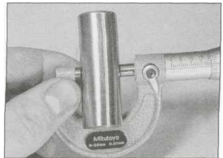
15.13b Measure the external diameter of the pin ...
