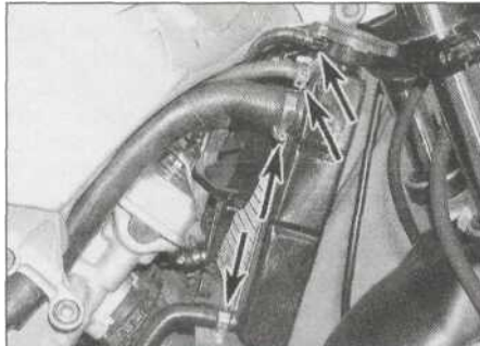
7.4a On YZF models, release the clamps (arrowed) and detach the hoses from the right-hand side ...
