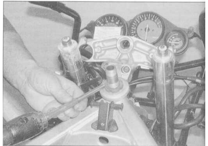
20.10 If the tool is not available, adjust the bearings as described
