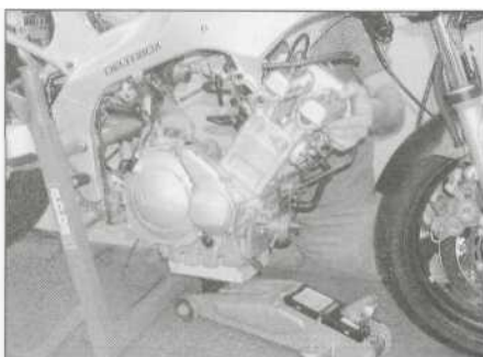
5.21 f Manoeuvre the engine out of the frame
