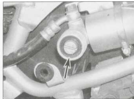
12.9 Compression damping adjuster (arrowed)
