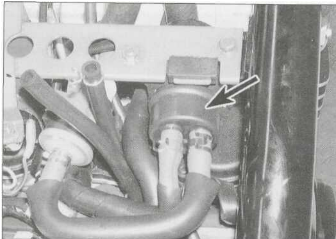
14.1c Fuel pump (arrowed) - FZS models
