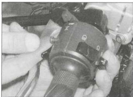
12.3a Remove the housing screws ,
