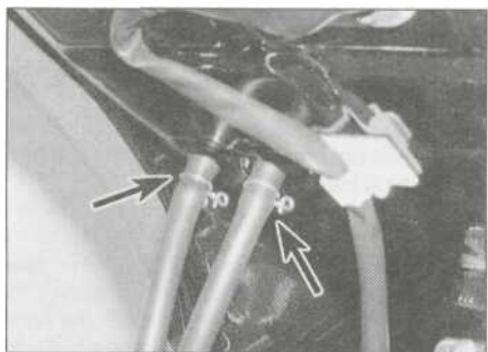
2.10a Detach the hoses, noting which fits where...
