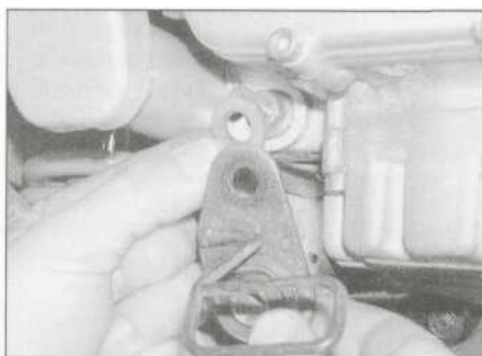
5.21 c Unscrew the nut and remove the bracket and washer
