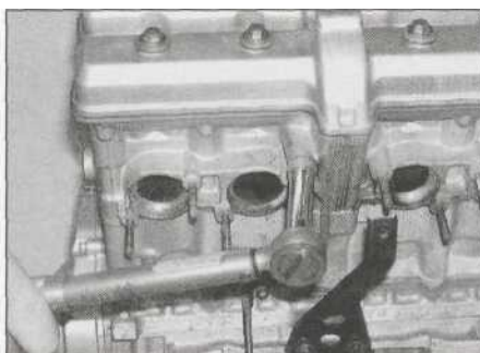
11.19b ... and tighten the bolts to the specified torque
