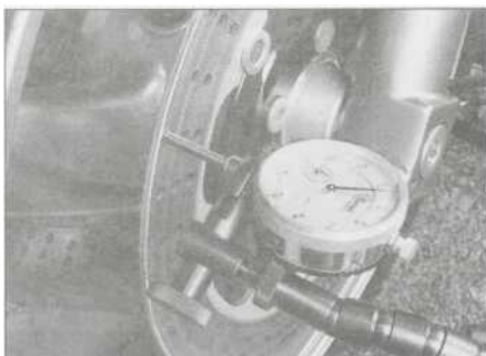
4.2 Set up a dial indicator with the probe contacting the brake disc, then rotate the wheel to check for runout
