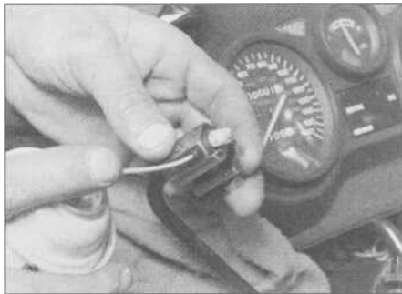
18.3a Lubricating a cable with a pressure lubricator. Make sure the tool seals around the inner cable
