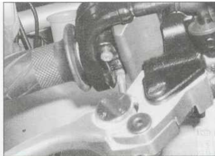
11.4b ... and remove the housing screws
