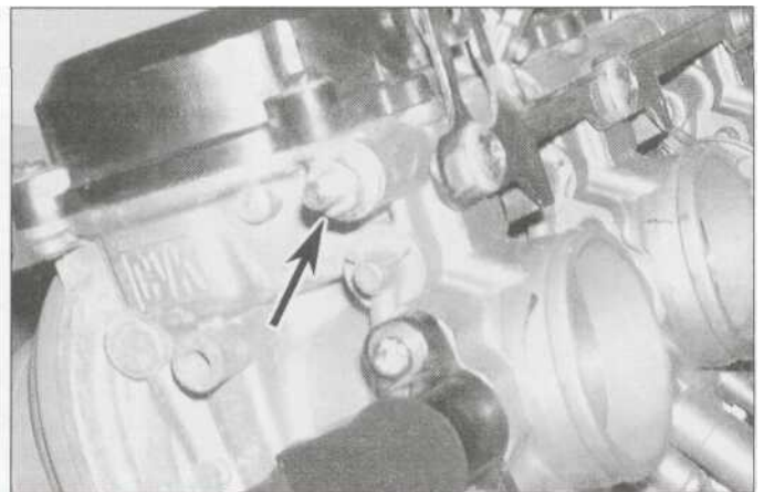
9.6a Unscrew the nut (arrowed) and withdraw the bolt...
