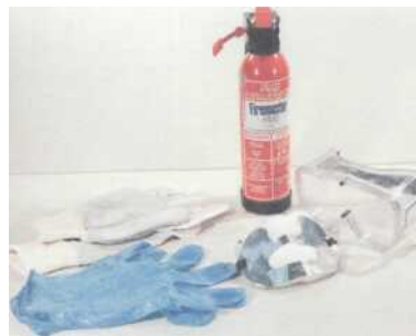
1.6 A fire extinguisher, goggles, mask and protective gloves should be at hand in the workshop
