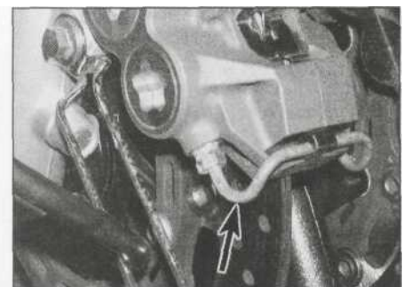
10.3 Check the condition of the metal pipe on each front caliper
