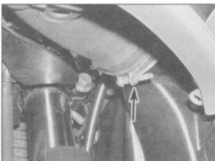
5.9a Slacken the front clamp (arrowed)...
