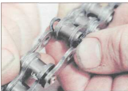
8.3 ... and separate the chain link
