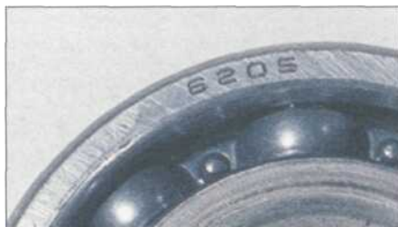
5.16 Typical bearing marking
