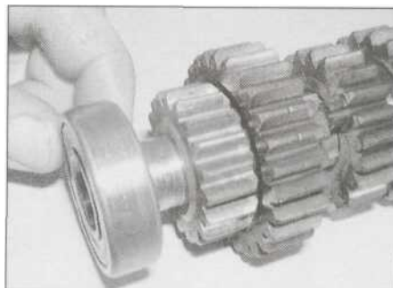
30.20 Fit the bearing onto the left-hand end of the shaft
