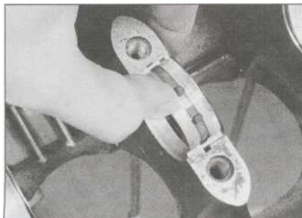
28.3 To remove a main bearing shell, push it sideways and lift it out
