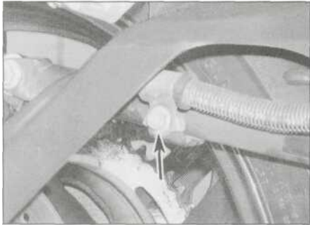
7.2a On YZF models, unscrew the bolt (arrowed) and free the brake hose
