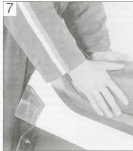
Bounce the rear of the motorcycle to check rear suspension operation
