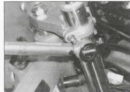
6.9c ... and the top yoke clamp bolt to the specified torque settings
