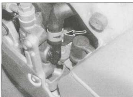
9.4b ... and detach the hose (arrowed) from the master cylinder
