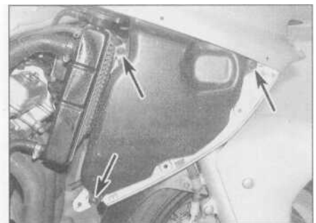
5.9c ... then remove the screws (arrowed) and detach the surge tank
