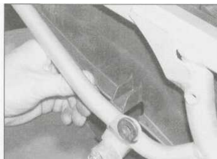
10.3f Push in the sides to free the mudguard from the frame ...
