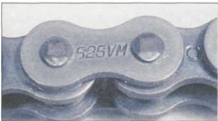
8.10 Typical chain size and type marking
