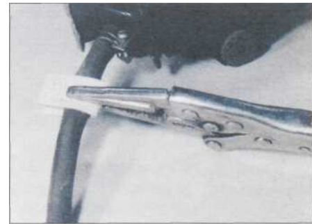
9.4 ... or thick card and self-locking grips
