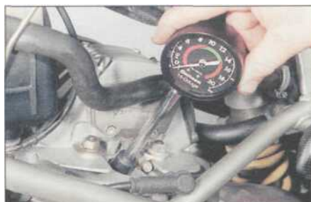
3.20 Using a rubber-cone type cylinder compression gauge
