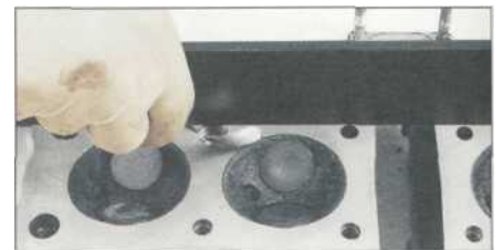
3.22 Use a straight-edge and feeler gauges to check for warpage
