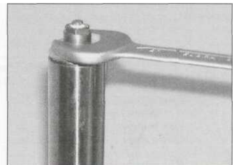
7.29 Thread the top bolt into the fork tube
