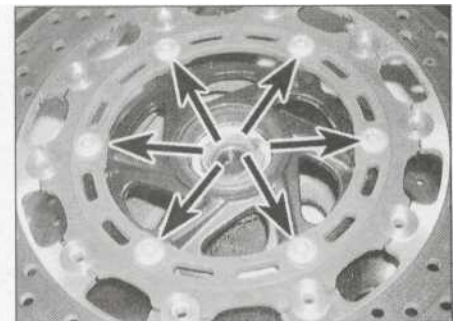
4.5 Unscrew the bolts (arrowed) and remove the disc
