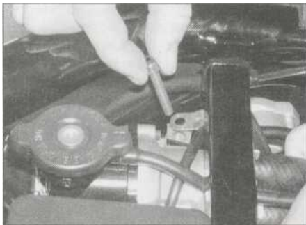
8.2a Unscrew the bolt securing the thermostat housing
