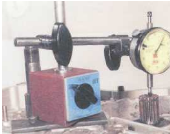
3.19 Using a dial gauge to measure shaft endfloat
