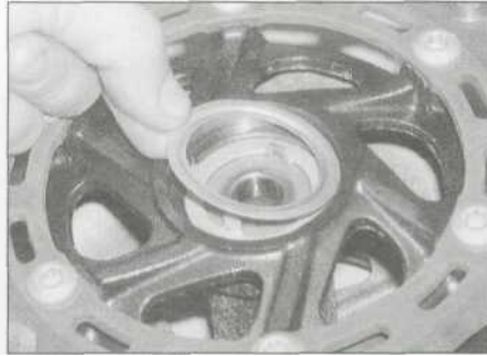
16.4b ... then lever out the retainer plate...
