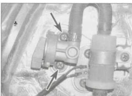
2.18a Fuel tap screws (arrowed)- YZF models
