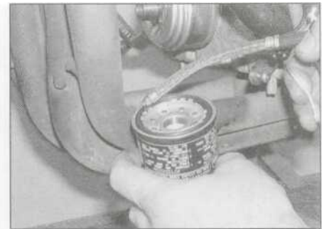
21.4a Smear some clean oil onto the seal..
