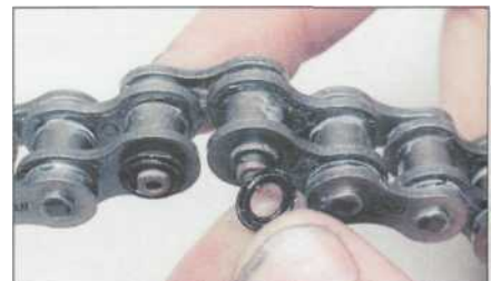
8.5 ... install the O-rings over the pin ends ...
