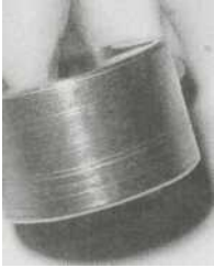
21.7 Look for scoring and wear, such as on this outer rotor
