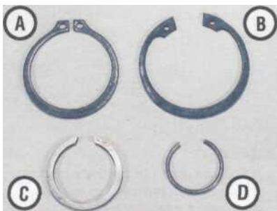
2.8 External stamped circlip (A), internal stamped circlip (B), machined circlip (C) and wire circlip (D)
