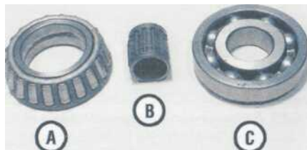
5.15 Tapered roller bearing (A), needle roller bearing (B) and ball journal bearing (C)
