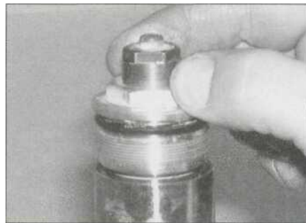
7.4 Unscrew the top bolt from the fork tube
