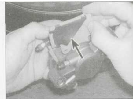
6.2e Remove the shim (arrowed) from the back of the pad, if one is fitted
