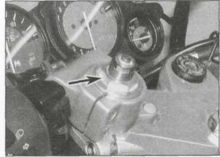
6.6b Slacken the top bolt (arrowed) if the forks are to be disassembled
