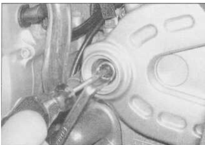
10.7b ... then slacken the locknut using a ring spanner and turn the adjuster using a screwdriver as described
