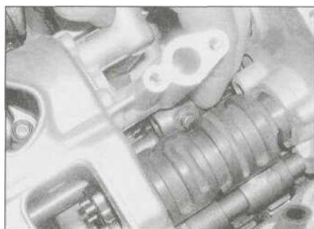
31.14 Position the fork against the drum so the guide pin is in the groove then slide the shaft through the fork
