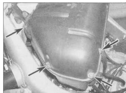
5.2a On YZF models, remove the four screws on each side (arrowed) and lift off the cover..
