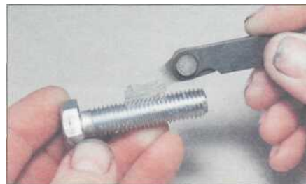
2.12 Using a thread gauge to measure pitch
