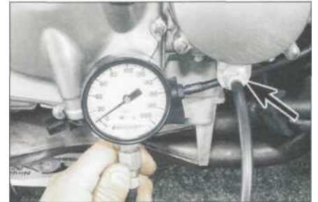
3.21 Oil pressure gauge and take-off point adapter (arrow)
