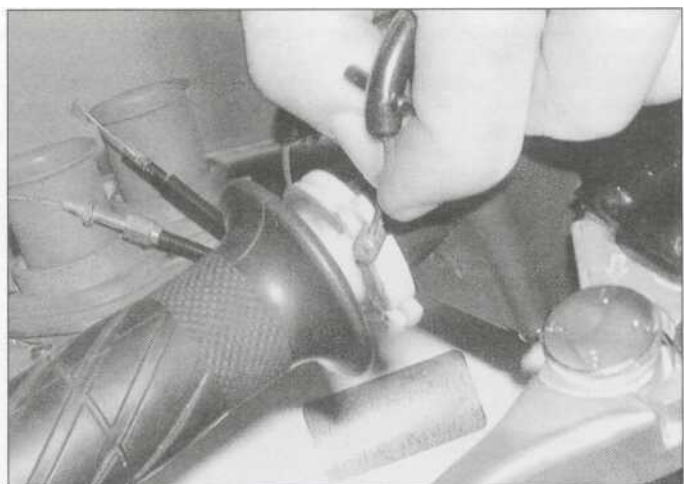
11.4d ... and free the cable ends from the throttle pulley
