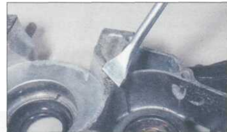
7.3 Paper gaskets can be scraped off with a gasket scraper tool...
