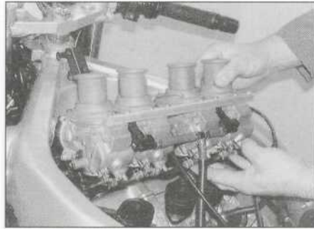
7.11d Draw the carburettors off the intakes and remove them
