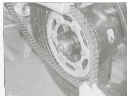
15.10 Manoeuvre the wheel into position and fit the chain onto the sprocket
