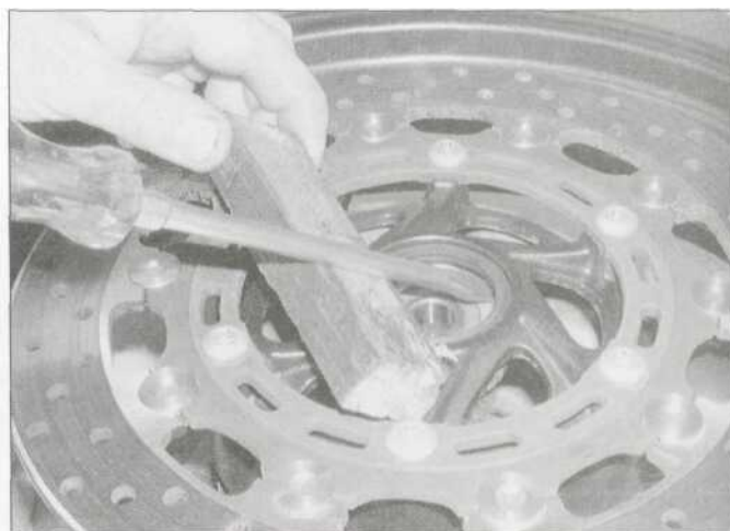
16.3 Lever out the grease seal
