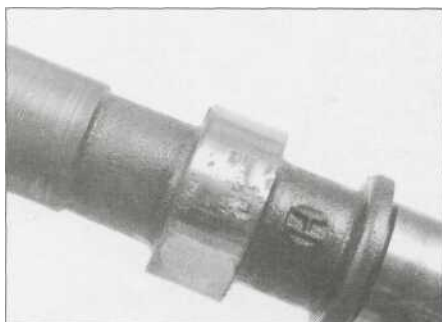
10.11 a Check the lobes of the camshaft for wear - here's an example of damage requiring camshaft repair or renewal
