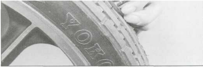
Checking the tyre tread depth
