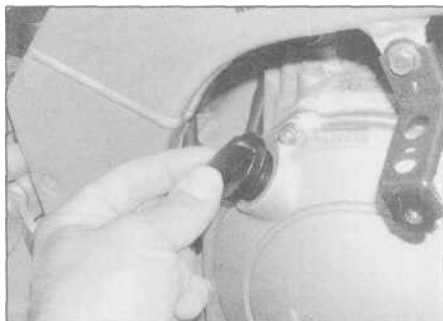
7.3 Remove the oil filler cap from the clutch cover
