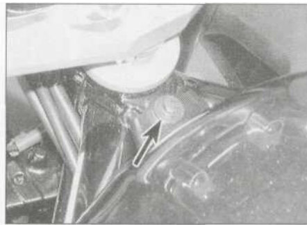
2.8b ... and remove the front bolt (arrowed)
