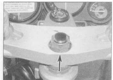
20.6b ... and unscrew the steering stem nut (arrowed)
