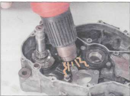
2.15 Using heat to free a seized fastener
