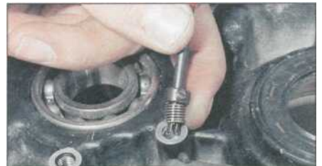
2.29 ... and thread into the component...
