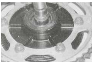
16.26a Use a socket to drive out the spacer...
