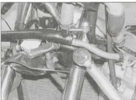
6.9a Tighten the bottom yoke clamp bolt..
