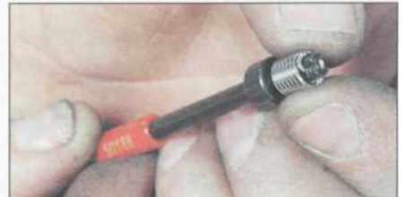
2.28 ... fit insert on the installing tool...
