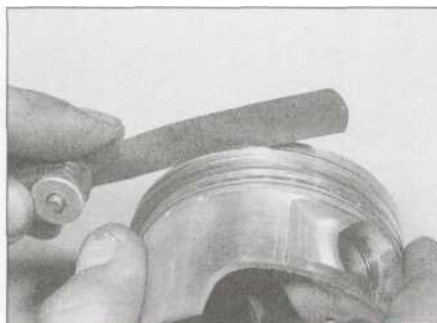
15.11 Measure the piston ring-to-groove clearance with a feeler gauge
