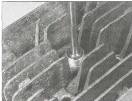
Installing a Helicoil thread insert in a cylinder head
