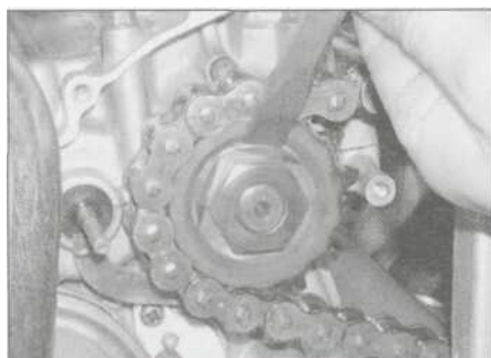
16.10d Bend the tabs up against the nut
