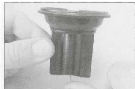
8.3c Push the needle up from the bottom and withdraw the holder and needle from the top
