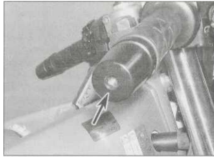
5.5 Unscrew the end-weight (arrowed) if required
