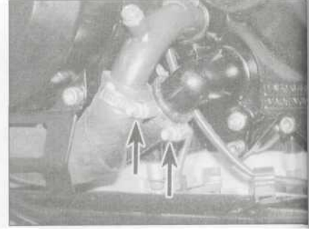
5.8c Slacken the clamps (arrowed) and detach the hoses, noting which fits where!
