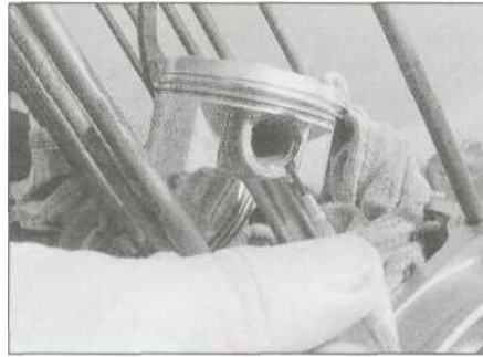
15.3a Prise out the circlip ..
