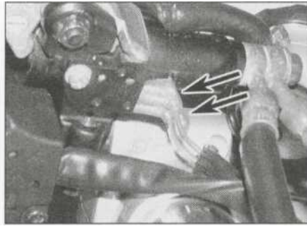
5.4 Brake switch wiring connectors (arrowed)
