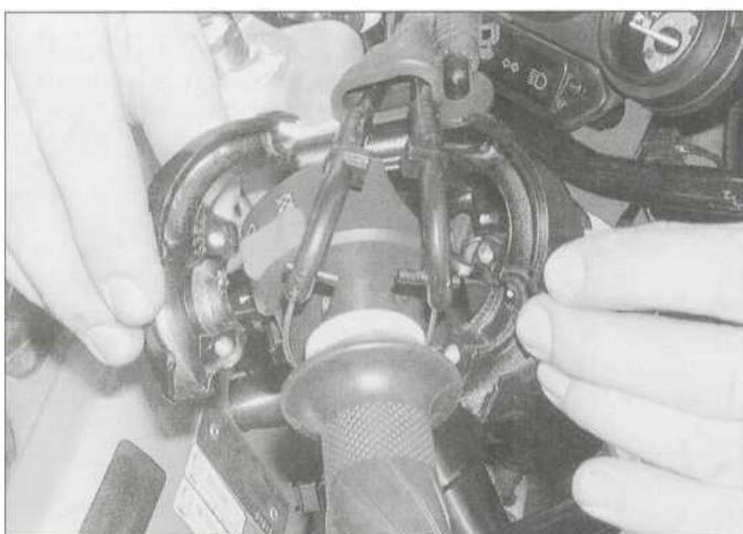
11.4c Separate the halves and detach the cable elbows ...
