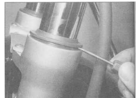
19.3a Lever off the dust seal...
