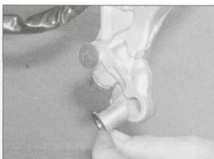
5.21 g Remove the collars from the left-hand front mounting
