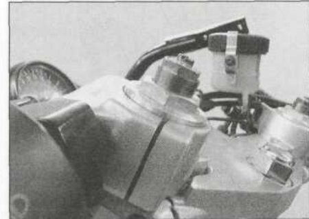
6.8 Align the top of the fork with the top of the handlebar holder on YZF model
