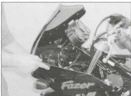
3.32 Carefully draw the fairing forward off the bike
