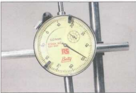
3.17 Dial gauge reading of 1.48 mm
