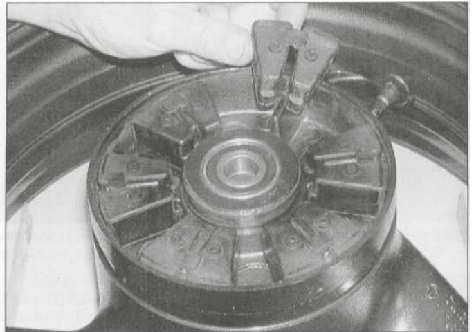
16.15b ... and remove the rubber damper segments
