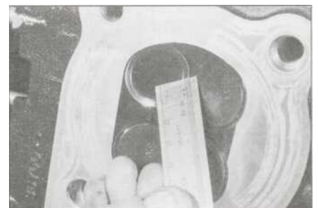
13.13 Measure the valve seat width with a ruler (or for greater precision use a vernier caliper)
