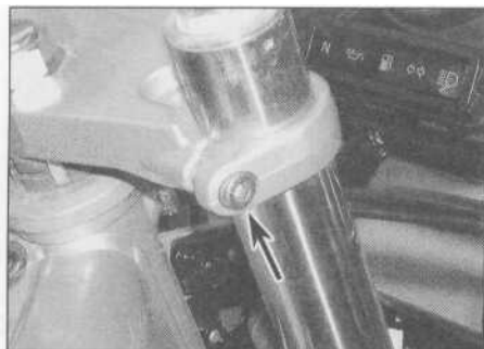
20.6a Slacken the fork clamp bolt (arrowed) on each side ...
