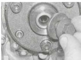
19.5 Unscrew the bolt and remove the washer
