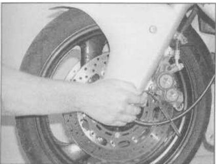
20.4 Checking for play in the steering head bearings
