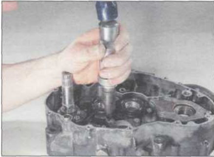
2.14 Using an impact driver to free a fastener
