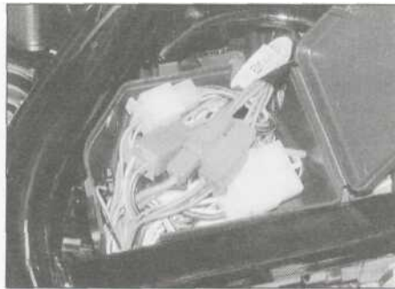
4.3b On FZS models, the fan motor wiring connector is in the connector box
