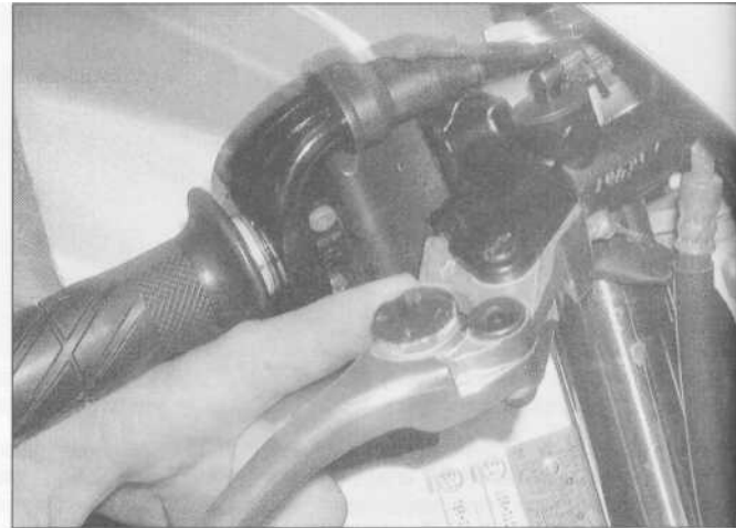
9.6 Front brake lever span adjuster
