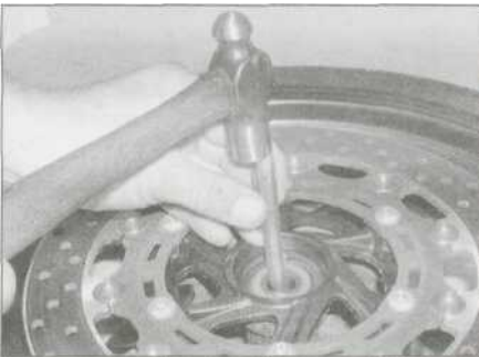
16.5a Knock out the bearings using a drift...
