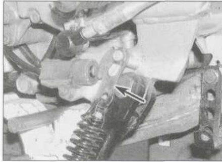
4.2a Unhook the springs and remove the hook plate (arrowed)...
