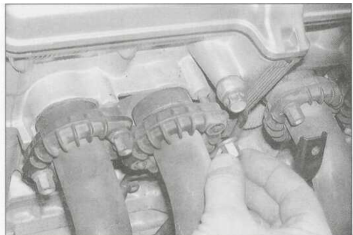
13.16 Fit the downpipe assembly nuts and tighten them to the specified torque
