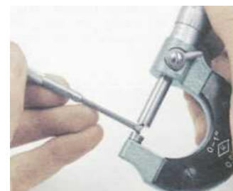
3.10 ... then measure the gauge with a micrometer
