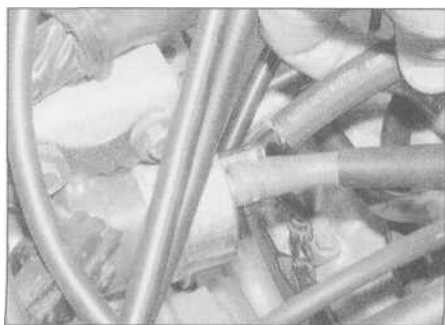
4.4c Connect the remote fuel supply to the fuel pump union
