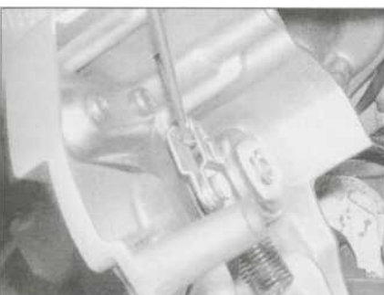
18.4a Bend down the retaining tab ...
