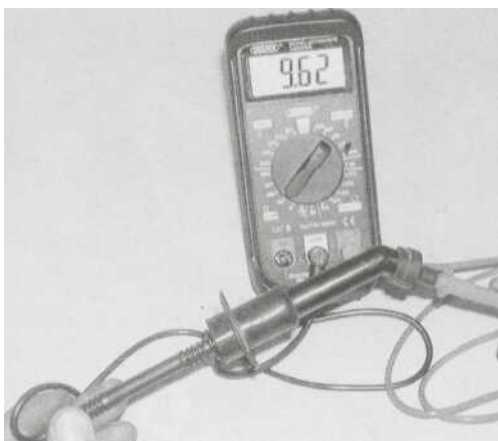
3.6 Measure the resistance of the spark plug cap
