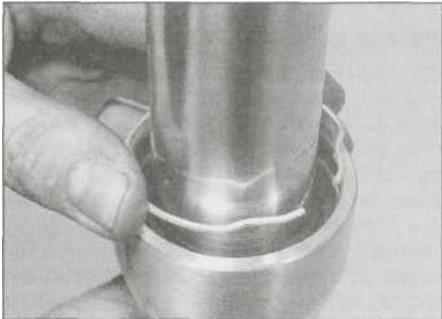
7.24 Install the retaining clip ...
