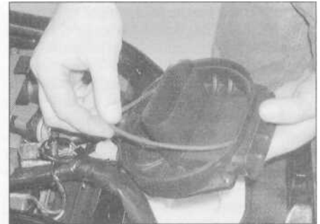
5.6b Make sure the rubber seal is in place - FZS shown
