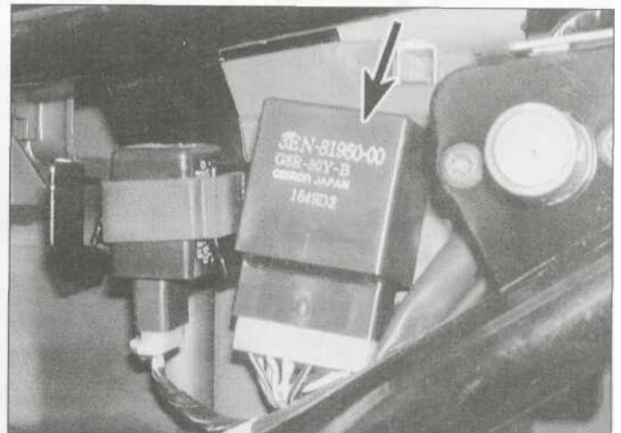
14.1d Relay (arrowed) • FZS models
