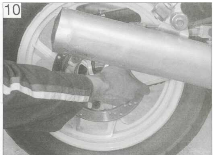
Grasp the swingarm at the ends to check for play in its pivot bearings
