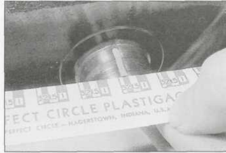
28.20 Measure the width of the crushed Plastigauge (be sure to use the correct scale - metric and imperial are included)
