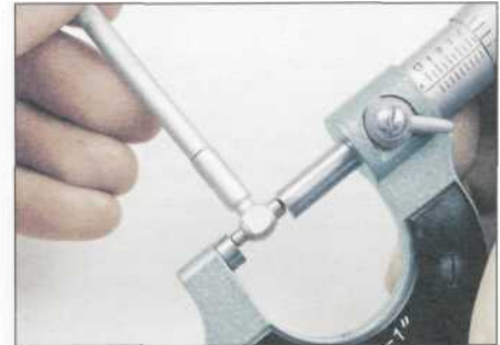
3.8 ... then measure the gauge with a micrometer
